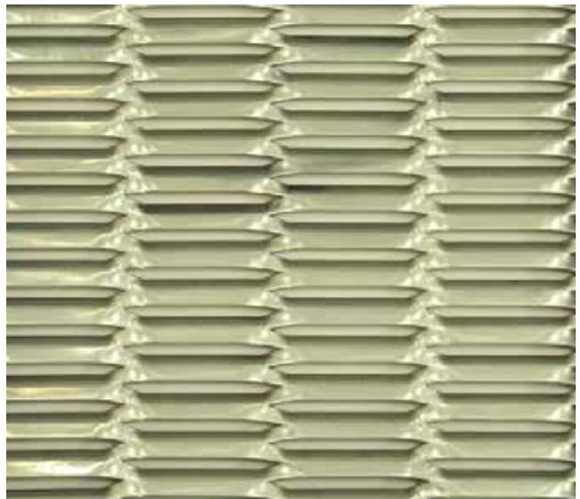
Expanded metal mesh as the name suggests is the process in which a plain sheet of stainless steel or aluminium is expanded by creating openings into the material through special dies which can vary in design as per customer requirements. This in turn results in the sheet to “expand” or elongate.
