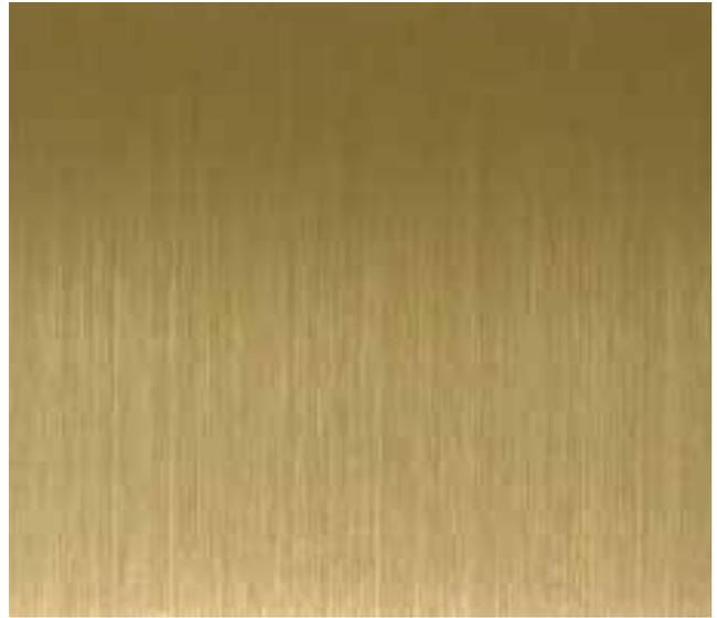
The name explains the look of the finish: these are well defined continuous uni-directional lines manufactured using abrasives that cut through the surface in microns. These differ from the #4 or Brush finish in surface roughness, grain structure and production methods. The Hairline finish is a smoother, reflective finish and is used primarily as a decorative product.
