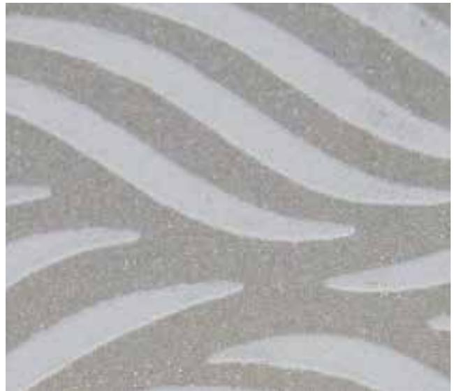
This finish is achieved using fine abrasives which are fired at the stainless steel in a stream of compressed air. This achieves a uniform, matt grey finish on components and fabricated parts such as castings. It can also be used selectively for decorative purposes
