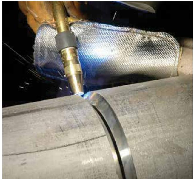
Cold Arc Weld - Welding with minimum heat input. Due to the minimum heat input, Cold Arc Weld is perfectly suitable for thin plates and heat sensitive materials such as Stainless Steel, Aluminium or high-strength steel. Cold Weld combines a pulsed arc with AC technology.
