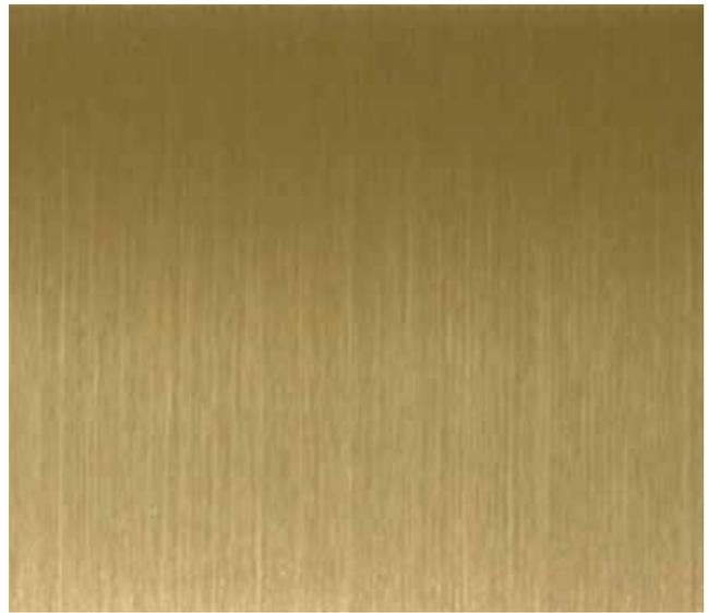
Also known as brushed, directional or satin finish. A #4 architectural finish is characterized by fine polishing grit lines that are uniform and directional in appearance. It is produced by polishing the metal with a 120–180 grit belt or wheel finish and then softened with an 80–120 grit greaseless compound or a medium non-woven abrasive belt
