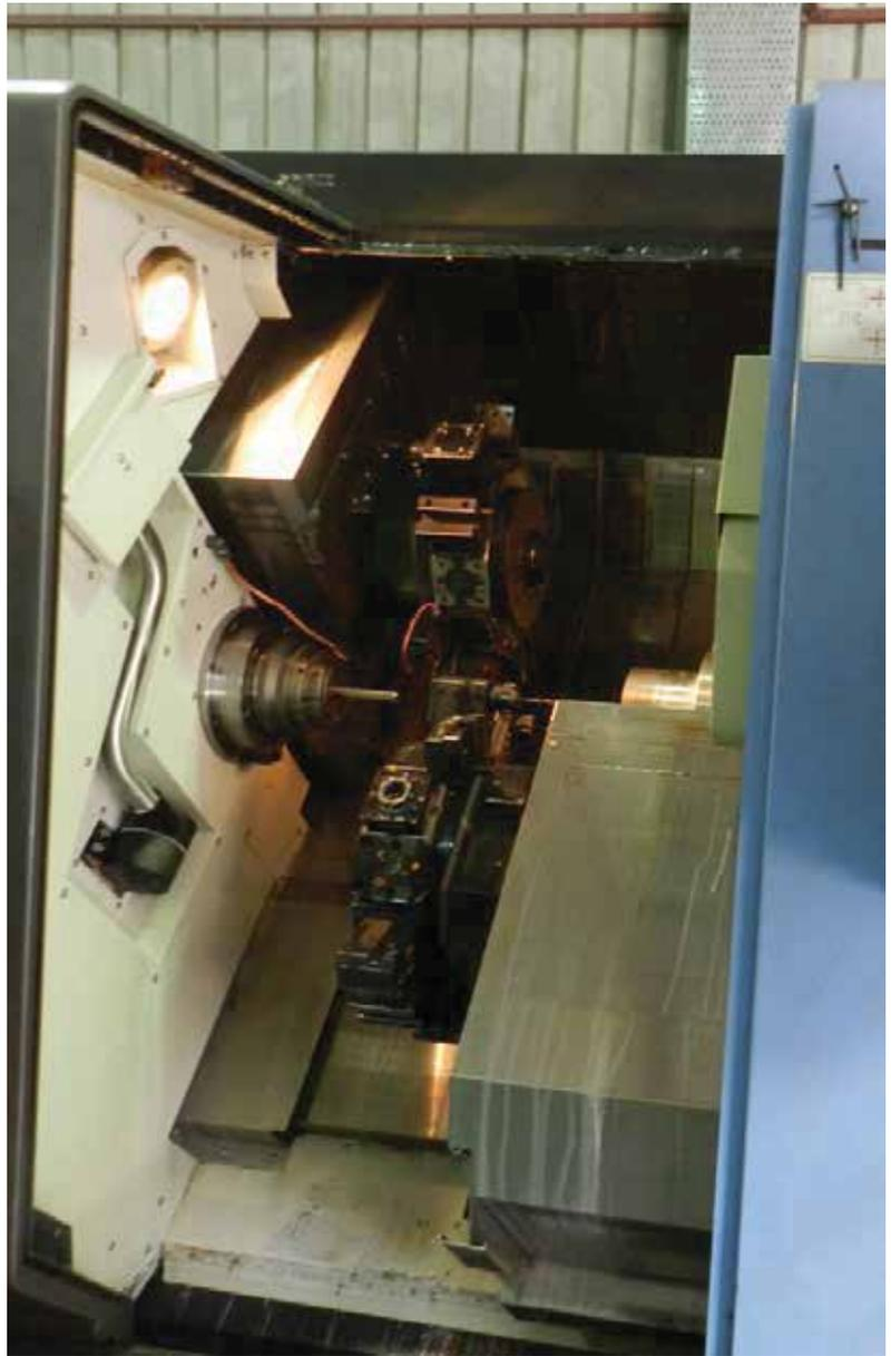
A lathe is a tool that rotates the work piece about an axis of rotation to perform various operations such as cutting, sanding, knurling, drilling, deformation, facing, turning, with tools that are applied to the work piece to create an object with symmetry about that axis. A chuck is a specialized type of clamp. It is used to hold an object with radial symmetry, especially a cylinder. On a lathe the chuck is mounted on the spindle which rotates.
