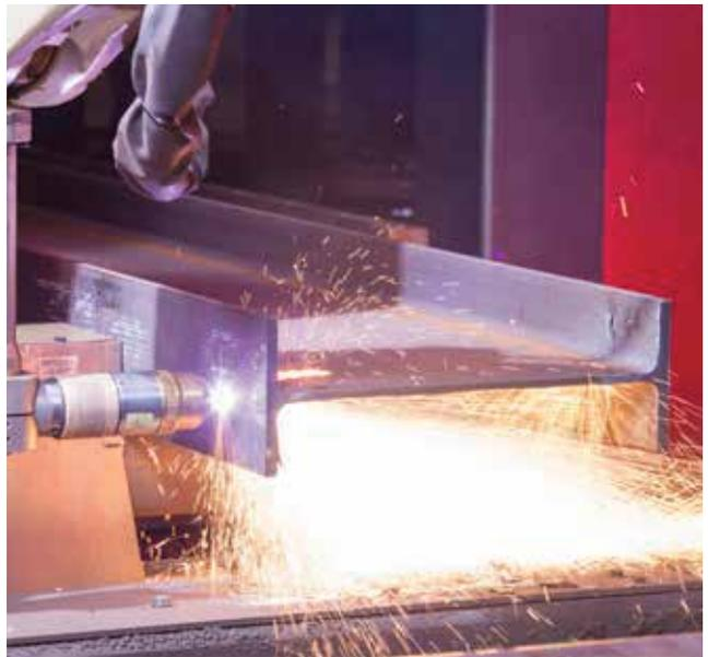
**Bolt Holes** – High quality, AISC compliant, in unlimited sizes with no tool changeovers; PythonX tilts the cutting torch, instantaneously changes speeds and uses sophisticated software to produce straight through holes that are nearly Taperless.
