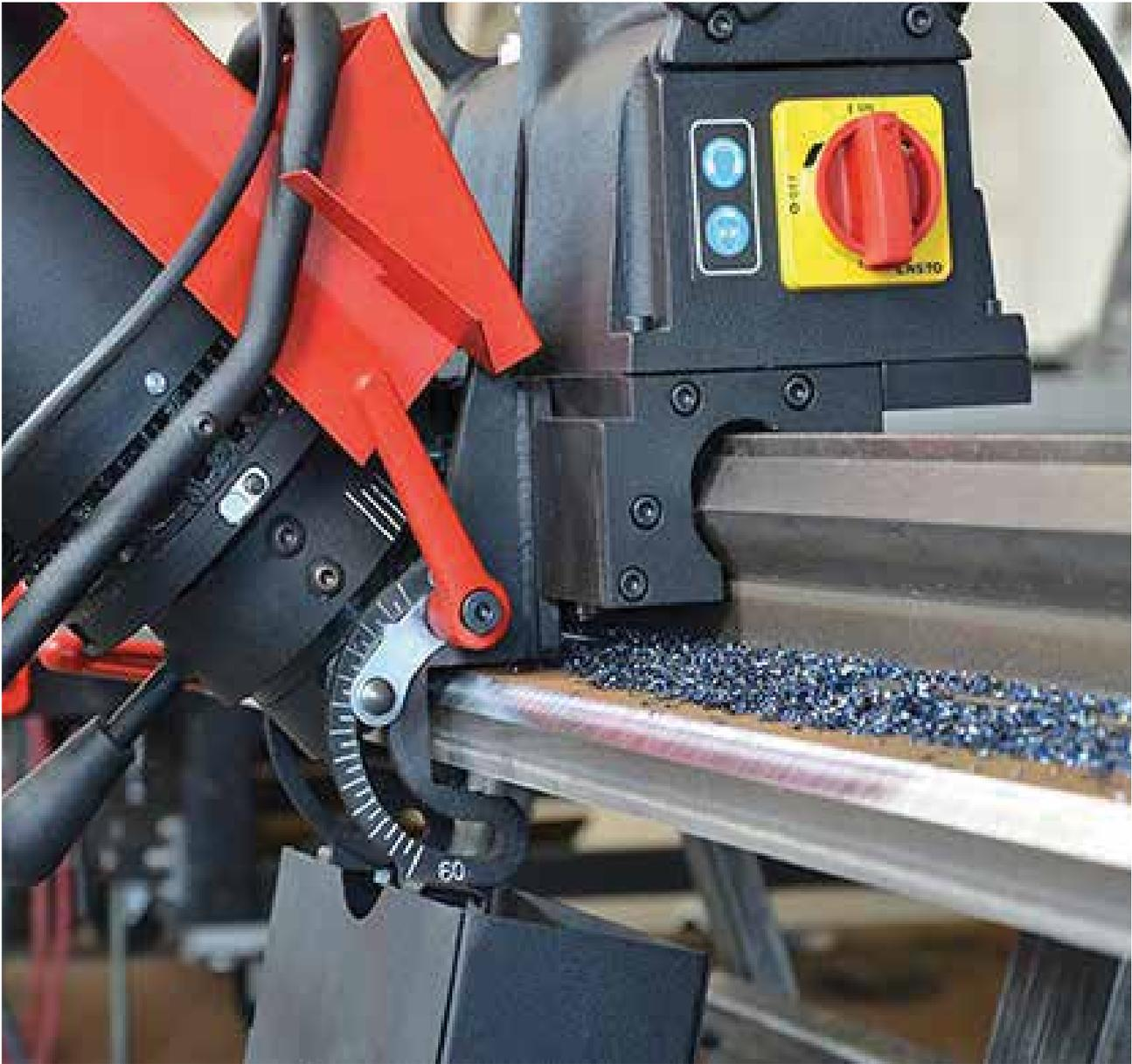
Simply put, a bevel is the angle that results from two meeting surfaces. A bevel cannot be at a 90° angle, but all other angles are acceptable as bevels.
