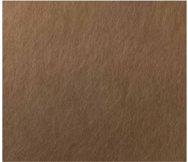
This is a non directional, non uniform finish made by vibrating rough abrasives that embed multiple continuous scratches overlapping each other. This is one of the popular finishes and could be called modern art on stainless steel.
