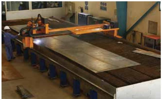
Plasma cutting is a process that cuts through electrically conductive materials by means of an accelerated jet of hot plasma. Plasma – a fourth state of matter which is ionized gas, it occurs when gas is heated at a very high temperature (20,000 deg. Cent.) And achieve equal number of positively charged ions and negatively charged ions. So under plasma cutting machine the gas is of high temperature and pressure. Thus it can only be used on high temperature and pressure.
