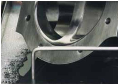
necessary to clean assemblies in between manufacturing steps to ensure contamination is not an issue. This can often be a problem when leading onto heat treatment or welding operations, as surface contaminants are easily absorbed into the upper surface layers and extremely difficult to remove.
